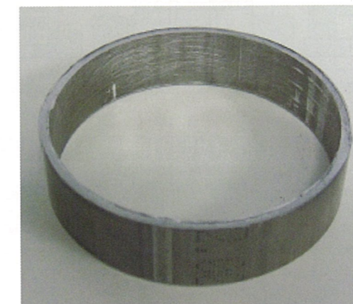
Figure 5b: Cutted steel tube (diameter 60 mm, thickness 2 mm).
