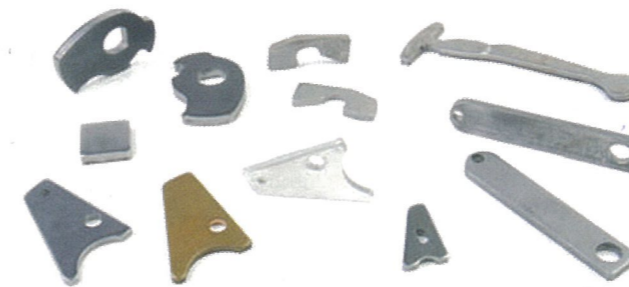
Figure 4: Example of blanked parts from different materials and shapes.
