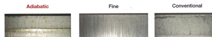
Figure 3: Blanked surfaces of steel part (4 mm thick): adiabatic, fine and conventional blanking [2].
