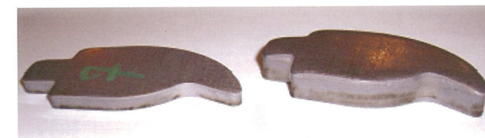
Figure 5a: Example of steel blanked parts: thicknesses 5 and 10 mm.
